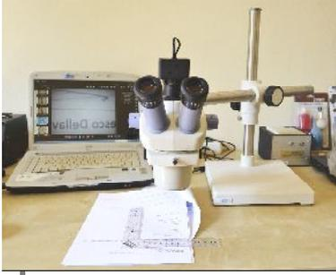
The kit that makes up the XTS 01 has been customized for document analysis, using a tilting stand for easy viewing of A / 3 - A / 4 format documents. Accessories: 5 Megapixel camera capable of operating in Truecolor and IR, lighting groups (NIR, UV), additional optics, bandpass filter wheel, reflex light polarization kit, solid state ring lighters, micrometer object on a slide, etc.
